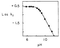
Figure 2. Plot of the logarithm of  $k_0$ , the buffer-independent rate constant for decomposition of potassium (E)-methanediazoate, as a function of pH at 25 °C, 1 M ionic strength (NaClO<sub>4</sub>).
